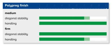
We recommend a **medium** or **firm Polypreg finish** for our **Fibercon® AP** cloth. The medium Polypreg finish is optimised for ease of handling, and the firm Polypreg finish for the diagonal stability needed in more performance oriented sails.
